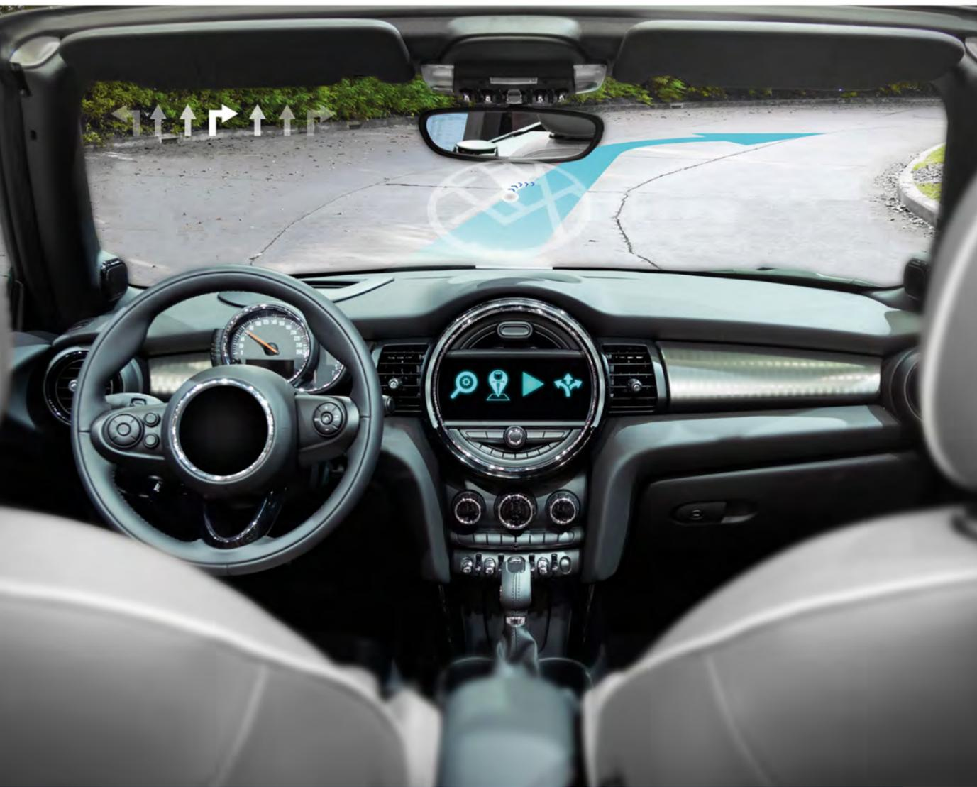
ple, a driver were to turn slightly and the system identified another vehicle ahead that was offset from the vehicle's own course, the AR Creator would have to pre-calculate the route ahead and tailor the virtual signals displayed accordingly. Due to the complex functioning of AR HUD, real-world test drives and conventional testing approaches are unsuitable for time-efficient and cost-efficient validation.
