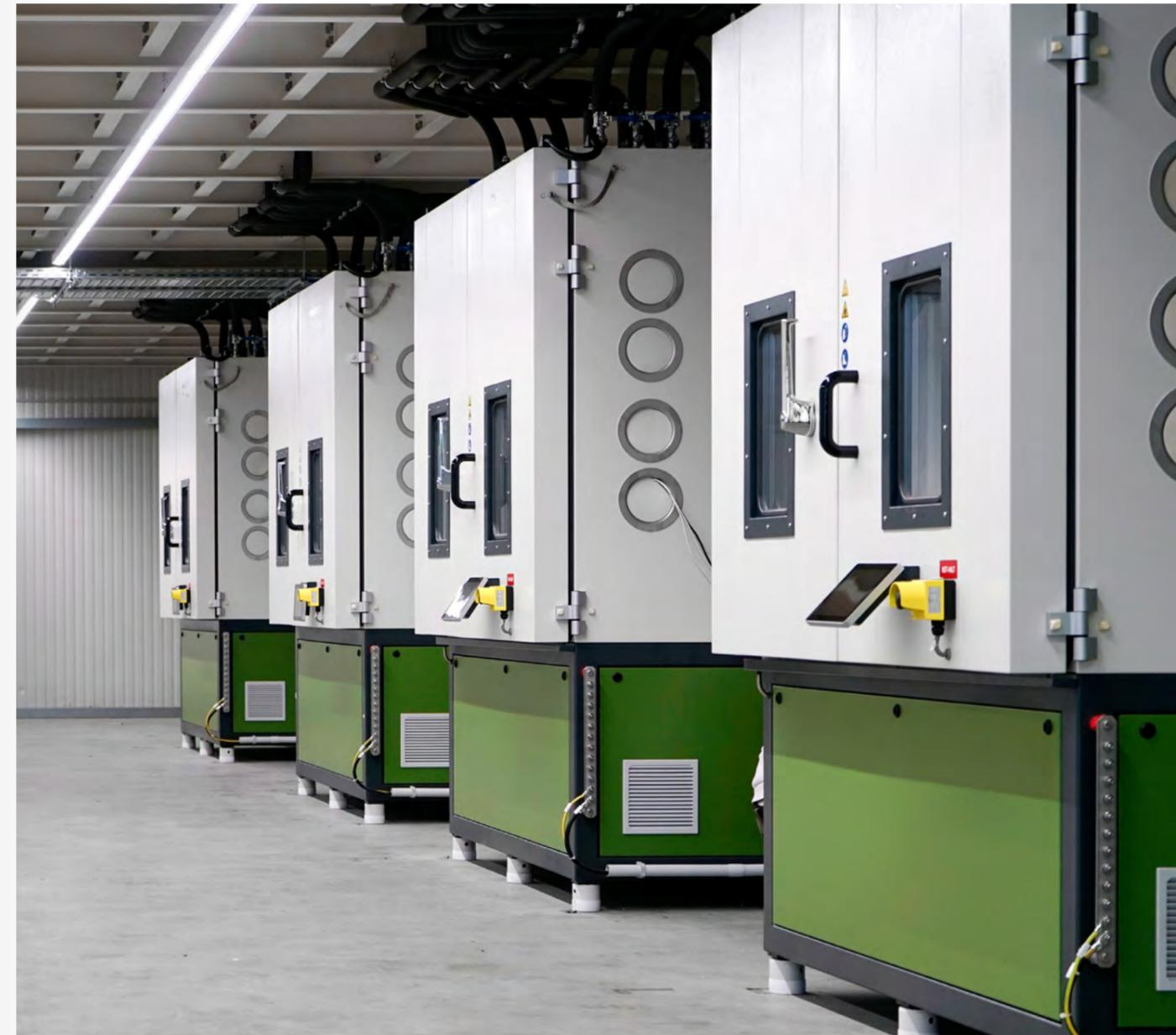
take care of all the process steps involved in component testing, including test reports, in ASAP's own laboratory. ASAP's service life simulation systems are safe, proven solutions. The systems' modular structure and use of STEP software enables the simple, swift and transparent integration of testing equipment, measurement technology and control technology, which ensures it is and will remain future-proof. They are desig-
